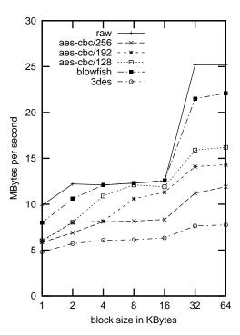
Figure 4: Throughput vs. block sizes of reads from the raw disk devices on P4 class machine
