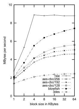
Figure 5: Throughput vs. block sizes of writes to the raw disk devices on ThinkPad 600E
